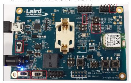
Figure 2: Switch and jumpers position
